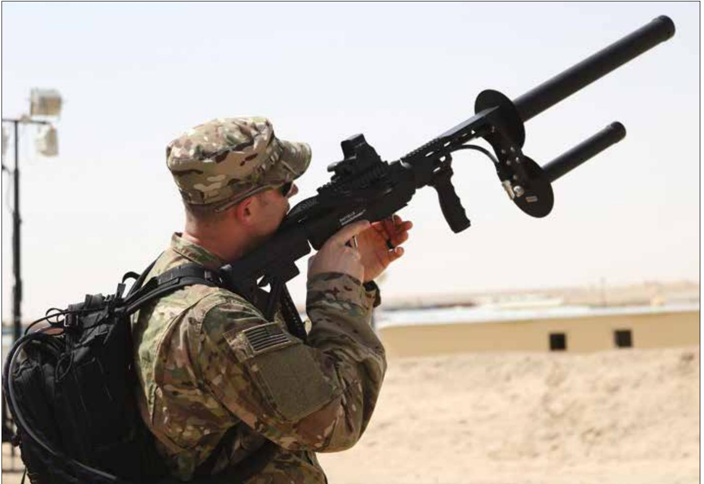
First Security Forces Assistance Brigade Soldier uses Drone Defender with electromagnetic pulse to disable, capture, and control target drone, Camp Buehring, Kuwait, March 6, 2018 (U.S. Army/Brent Thacker)
